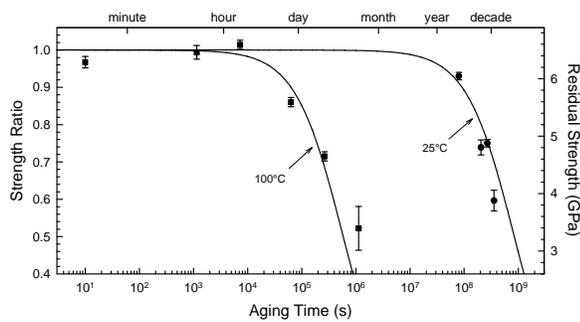
**Fig. 1** Residual strength of fused silica optical fibre after aging under zero stress in distilled water
