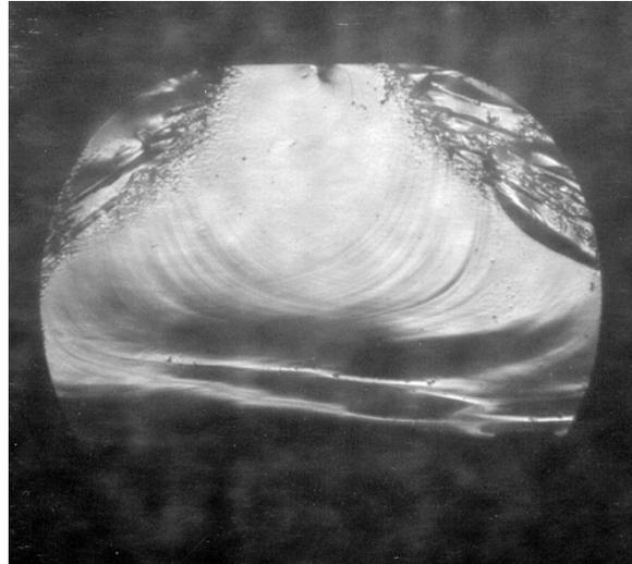
Fig. 3. Fracture surface of indented flat fiber.
