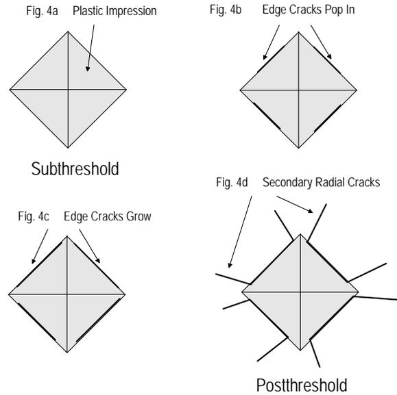
Fig. 4. Pop in sequence for dry N<sub>2</sub> indentation.
