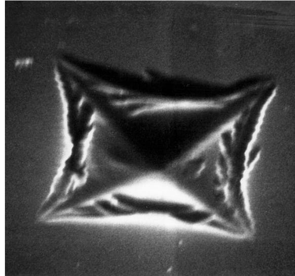
Fig. 10. SEM image of 50 mN indentation aged 4 weeks in 90°C pH 7 buffer (8000X).
