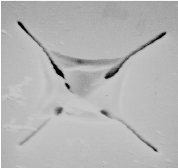
Fig. 9. SEM image of 25 mN indent aged 4 weeks in 90°C pH 7 buffer with radial cracks (8000X).
