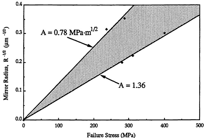
**Figure 7.** Transformed mirror radius as a function of failure stress.
