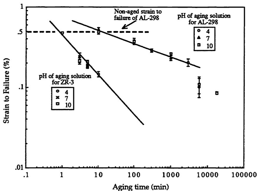
**Figure 4.** Effect of zero-stress aging of coated fibers on strain to failure at 80°C.
