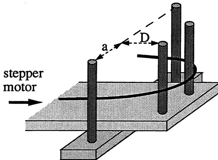
Figure 1. Four-point bend apparatus.
