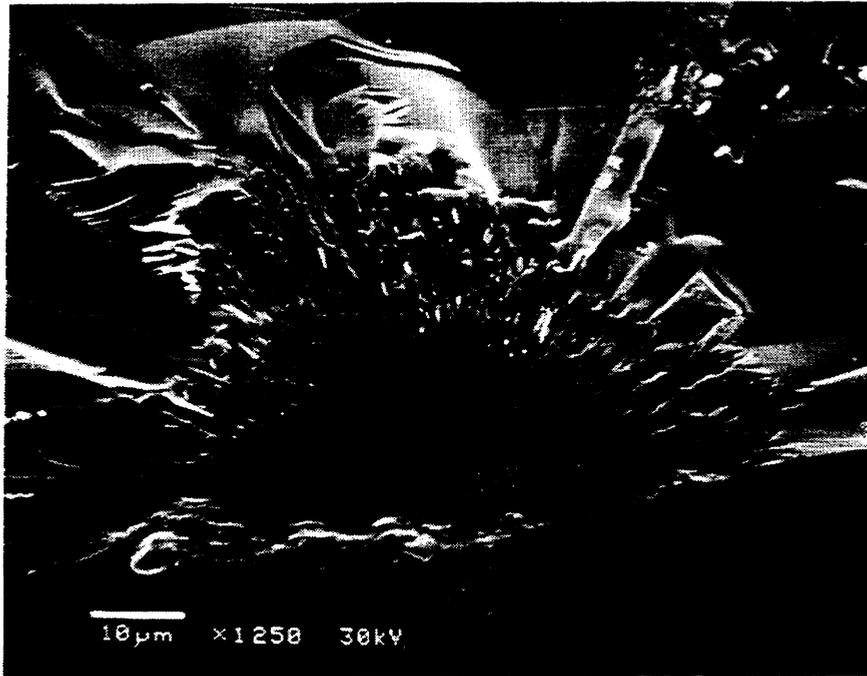
**Figure 2.** Fracture surface of aluminum fluoride-based glass fiber, showing mirror zone.
