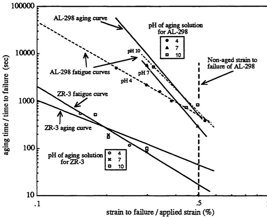
Figure 6. Comparison of static fatigue and zero-stress aging curves.
