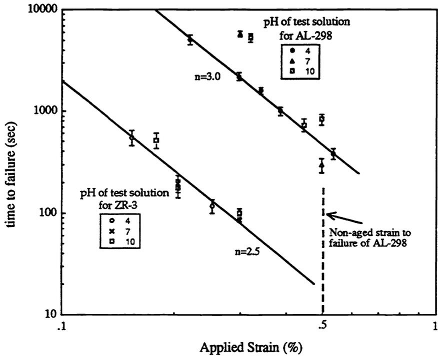
Figure 5. Effect of strain on time to failure at 80°C.
