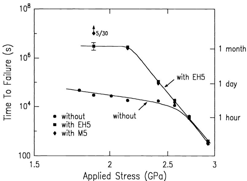
Fig. 3. Static fatigue in 90°C pH 7 buffer solution of fiber without any coating additive and with 3 wt% of grades M5 and EH5 colloidal silica particles in the coating.<sup>33</sup>
