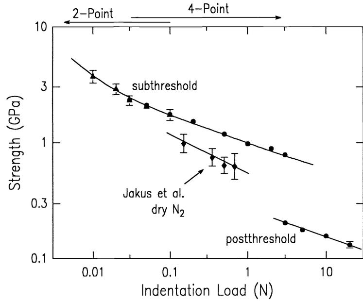
Fig. 1. Inert (liquid nitrogen) strength of indented fiber as a function of indentation load as measured by two and four point bending (after Ref. 17).
