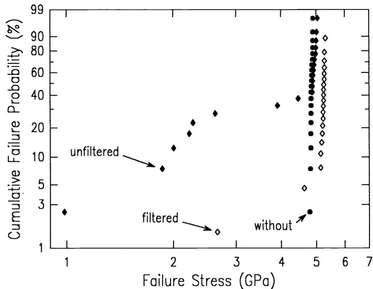
Fig. 4. Weibull probability plot of the tensile strength (300 mm gauge length) of fiber without silica particles in the coating, and fiber with 3 wt% of M5 particles in the coating when the liquid prepolymer has been both unfiltered and filtered through a  $20 \mu\text{m}$  membrane (after Ref. 33).
