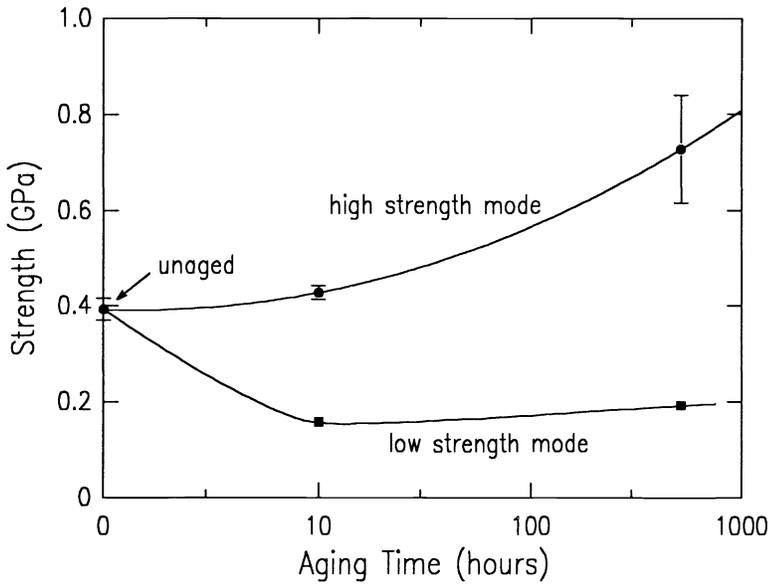
Fig. 2. Residual strength (measured by two-point bending in 27°C pH 7 buffer) of fiber indented at 0.5N, as a function of aging time in 90°C pH 7 buffer.<sup>17</sup>
