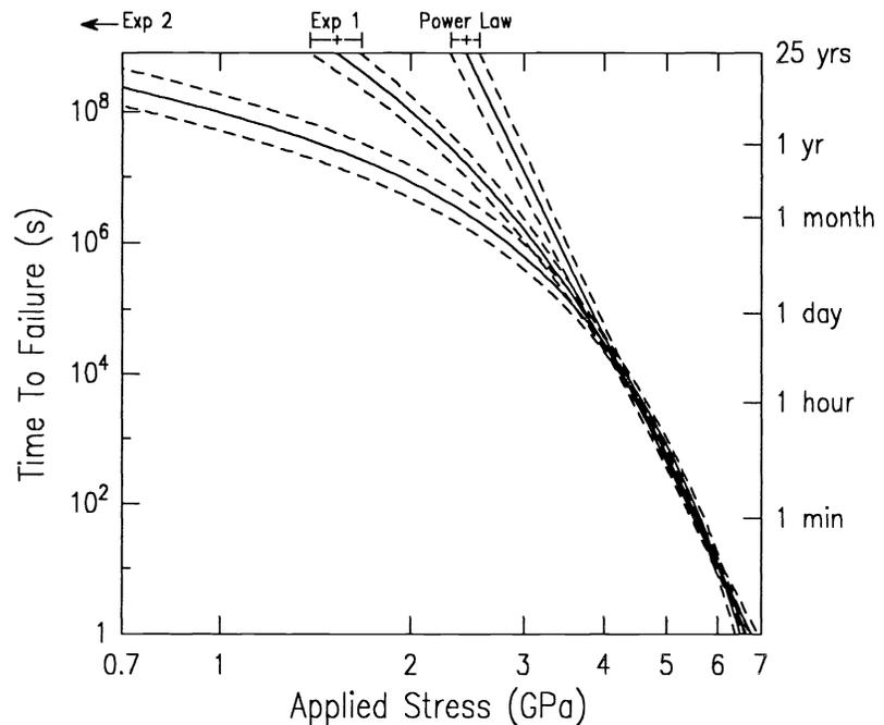
Fig. 5. Extrapolation of short term fatigue data to a 25 year lifetime for measurements made in 25°C air.<sup>42</sup>
