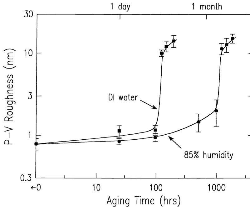
Fig. 4. Peak to valley roughness (measured from 1.5  $\mu\text{m}$  square AFM scans) as a function of aging time under zero stress in 85°C (■) deionized water and (●) 85% relative humidity.
