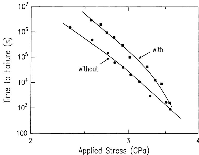
Fig. 5. Static fatigue data measured in two-point bending and a 85°C, 85% relative humidity environment for fiber both with (■) and without (●) ~0.7 wt% of colloidal silica incorporated in the polymer coating.
