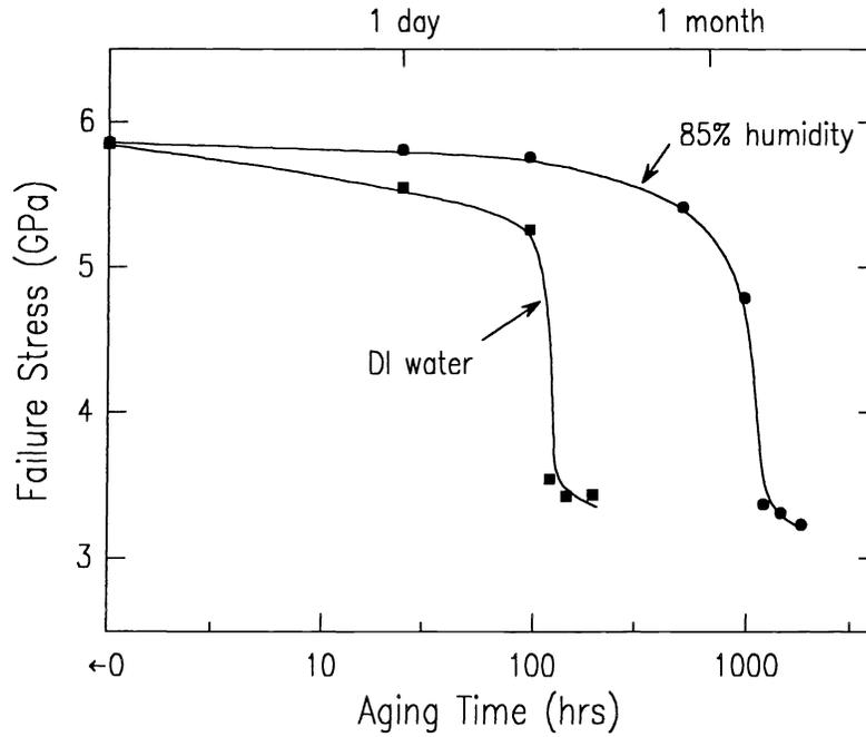
Fig. 3. Residual strength, measured in two-point bending in 23°C, 50% relative humidity, as a function of aging time in 85°C (■) deionized water and (●) 85% relative humidity.
