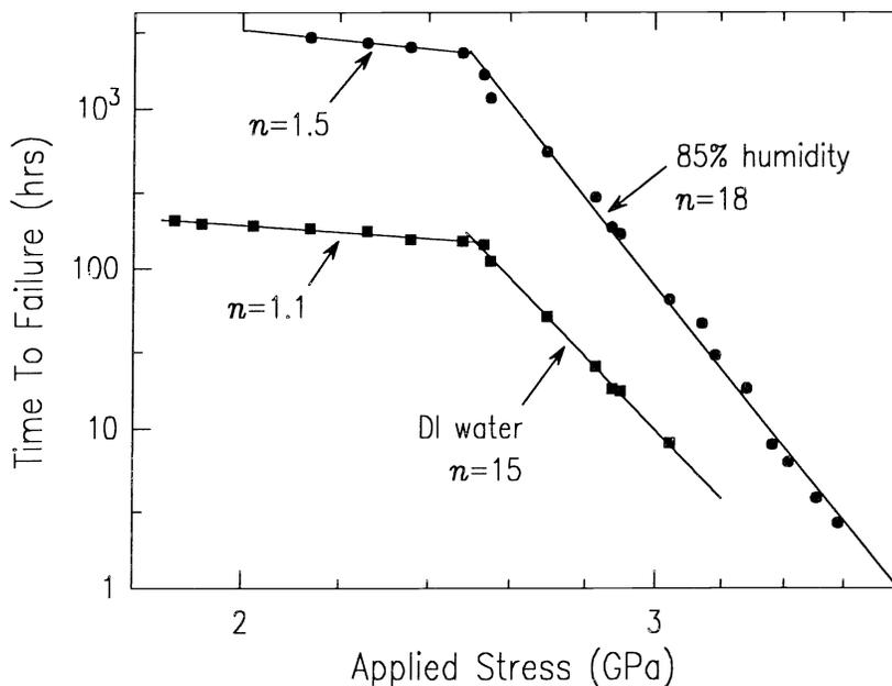
Fig. 2. Two-point static fatigue of fiber in  $85^\circ\text{C}$  (■) deionized water and (●) 85% relative humidity.
