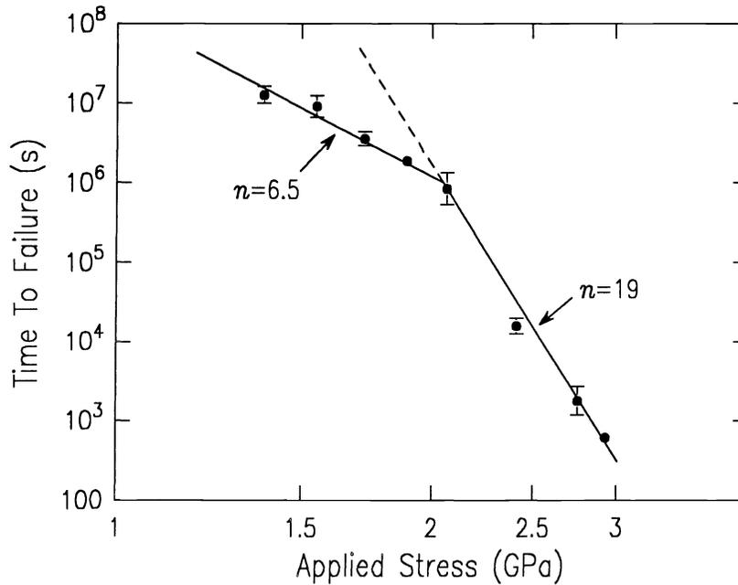
Fig. 1. Tensile static fatigue data for laser drawn TO-8 clad fiber tested in 32.6°C 90% relative humidity (after Wang and Zupko<sup>1</sup>).
