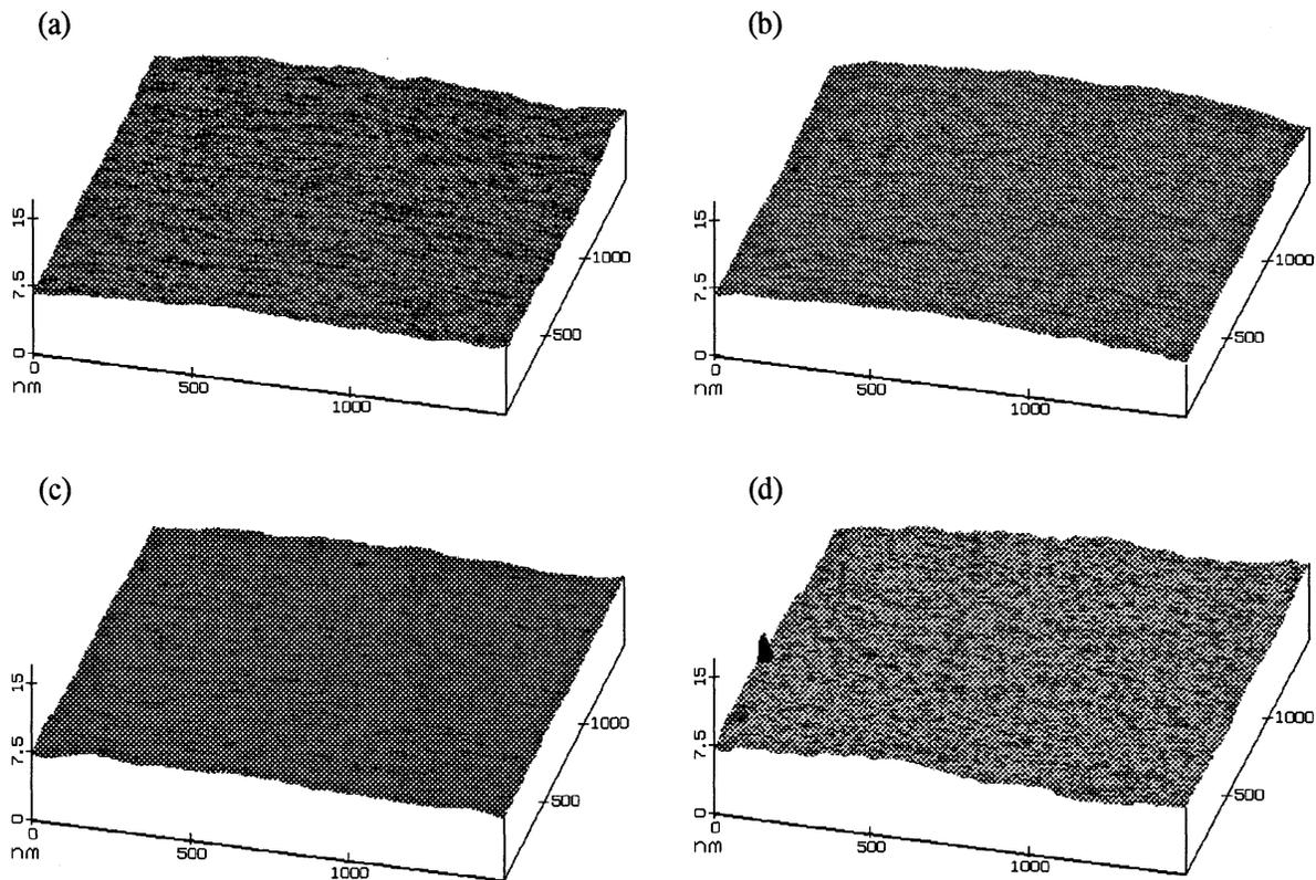
Fig. 1. AFM profiles of the bare fiber surface of fibers (a) A, (b) C, (c) D and (d) E, stripped in 40°C FeCl<sub>3</sub> for 10 minutes.
