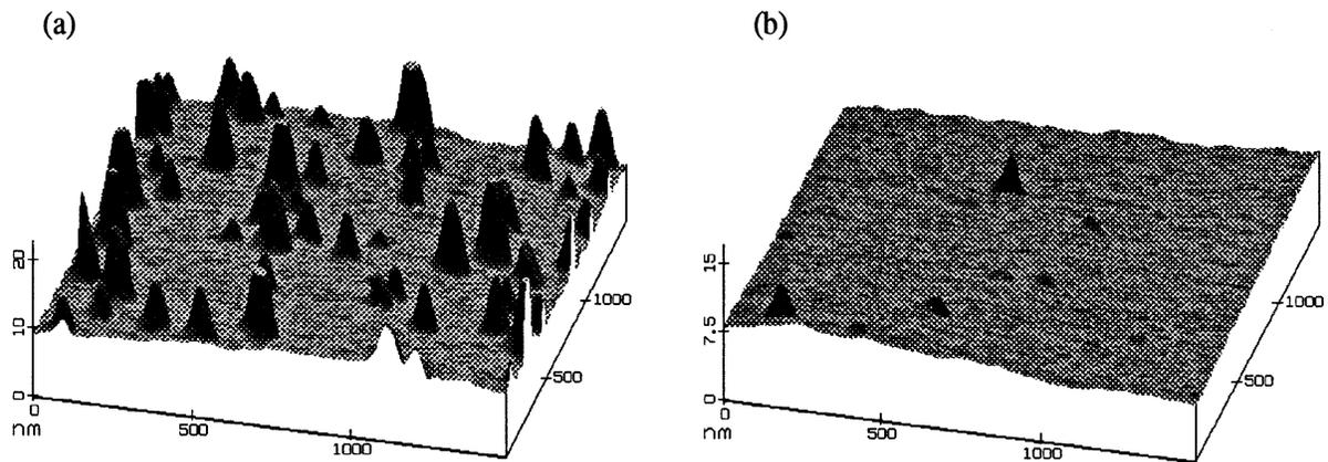
Fig. 2. AFM profiles of the bare surface of fiber B after stripped in 40°C FeCl<sub>3</sub> for (a) 10 minutes and (b) 20 minutes.
