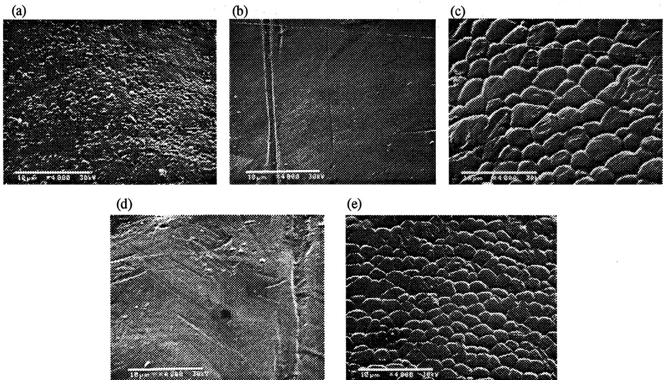
Fig. 3. SEM images of the aluminum surface of fibers (a) A, (b) B, (c) C, (d) D and (e) E. Scale bars are 10 μm long.
