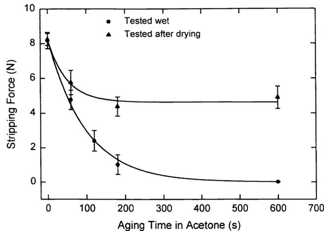
**Figure 8.** Stripping force of fiber as a function of immersion time acetone.
