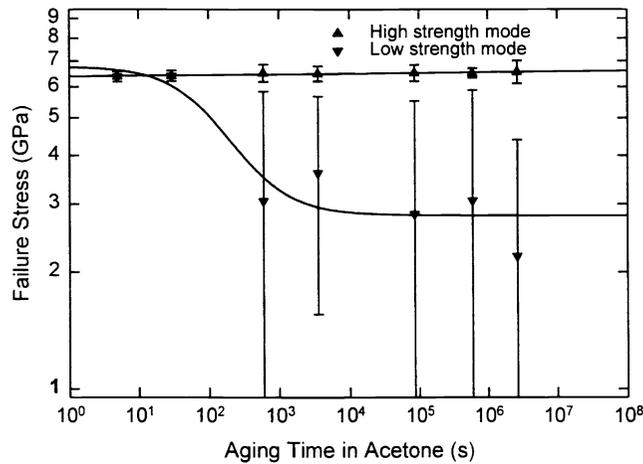
**Figure 7.** Bimodal residual strength of fiber measured in bending as a function of aging time in acetone.
