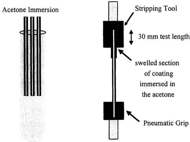
Figure 3. Schematic of stripping force experimental set-up.
