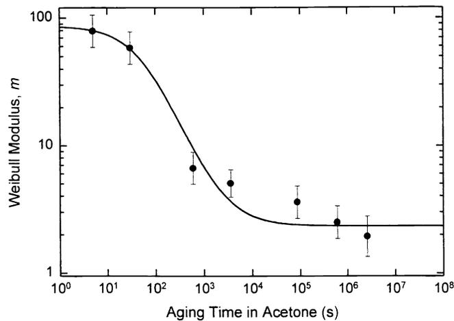
**Figure 6.** Weibull modulus,  $m$ , of fiber measured in bending as a function of aging time in acetone.
