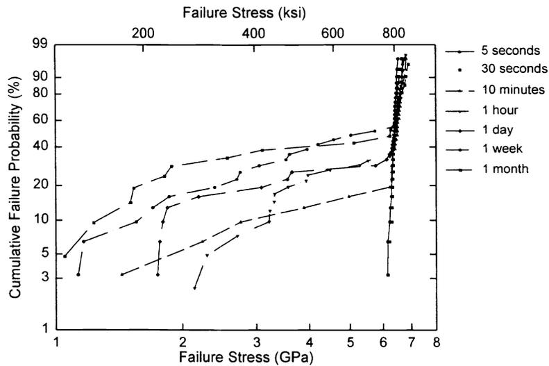
Figure 5. Weibull plot of the bending strengths of fibers soaked for various times in acetone.
