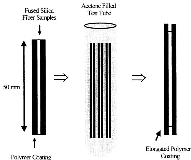
**Figure 1.** Schematic of sample preparation for bending measurements.
