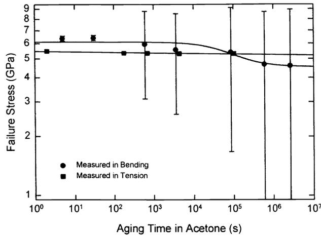
Figure 4. Two-point bending and tensile strength as a function of soak time in acetone.
