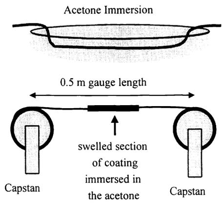
Figure 2. Schematic of tensile experimental set-up.
