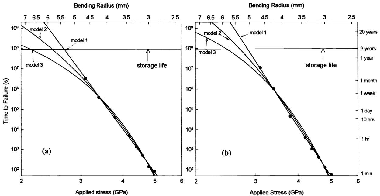
Figure 4. Static fatigue data of (a) fiber I (b) fiber II fitting to various kinetics models.
