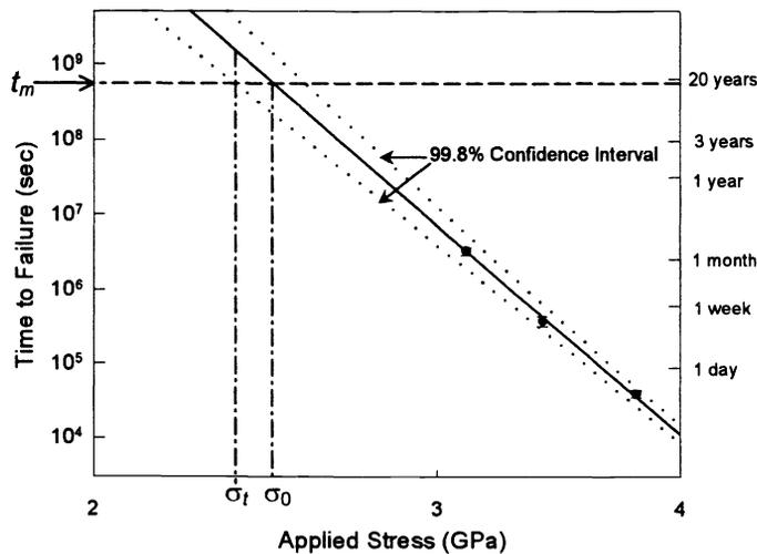
Figure 3. Extrapolation of static fatigue data of fiber I (detailed from figure 1) to the median failure time and the corresponding stress to lower confidence bound.
