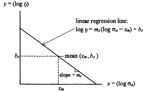
Figure 2. Schematic of linear regression model for fitting static fatigue data.
