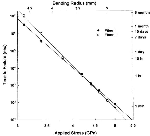
Figure 1. Static fatigue data for fiber I and fiber II measured in 30°C pH7 buffer solution.
