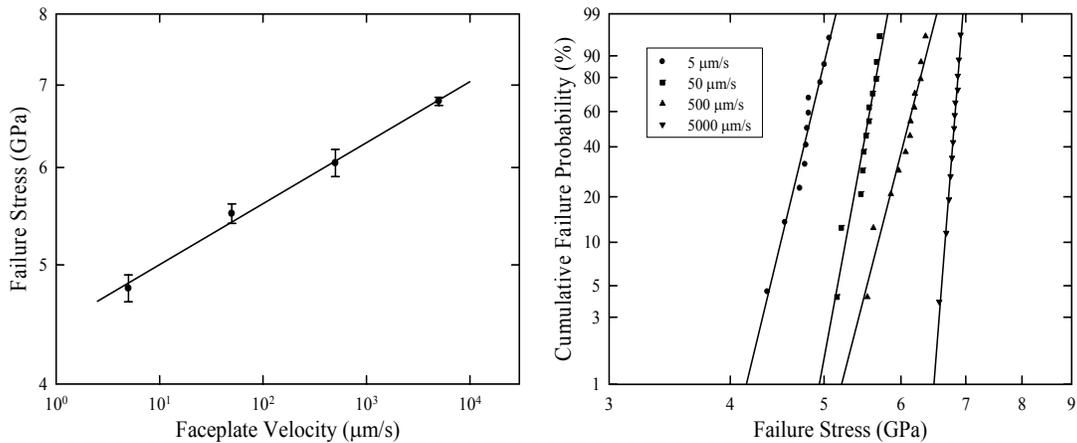
Fig. 1. Dynamic fatigue and Weibull plots of the bending strength for fiber with a single coat of HG-4
