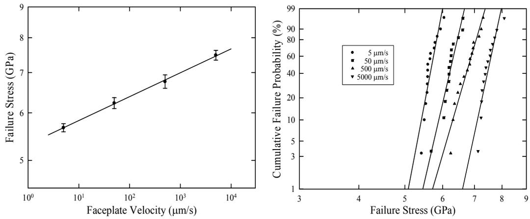
Fig. 2. Dynamic fatigue and Weibull plots of the bending strength of fiber with dual coats of HG-4
