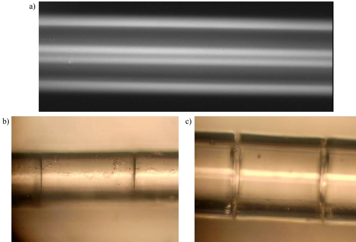
Fig. 5. Optical microscope images of (a) fiber 1 with single coat of HG-4, (b) fiber 3 with a single layer of HG-4MP, and (c) fiber 4 with dual coat of HG-4MP.
