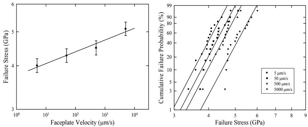
Fig. 3. Dynamic fatigue and Weibull plots of the bending strength of fiber with a single coat of HG-4 MP
