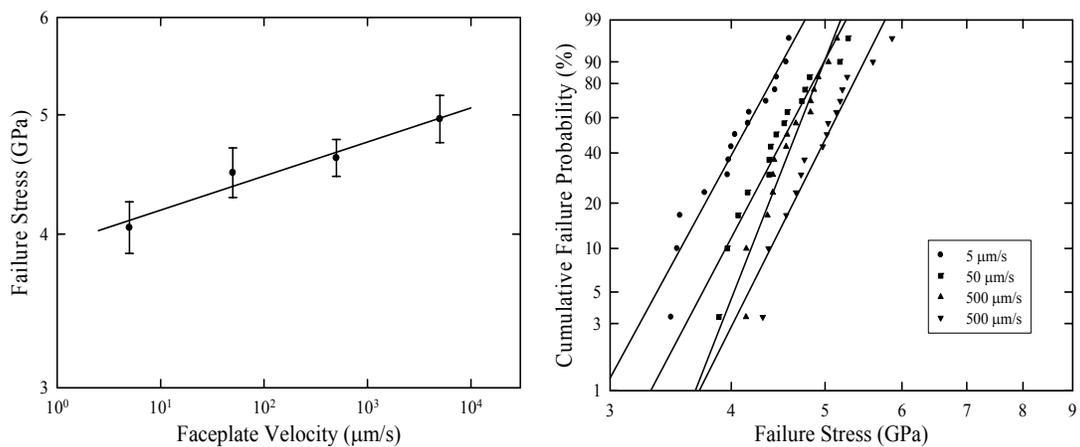
Fig. 4. Dynamic fatigue and Weibull plots of the bending strength for fiber with a single coat of HG-4MP that was heat cured online in addition to the UV cure.
