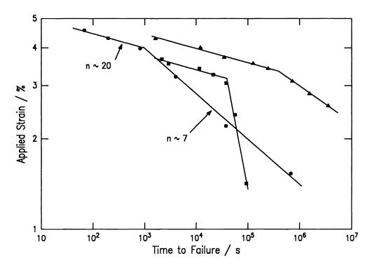
Fig. 1. Static fatigue results for fiber tested in tension. Key: • bare fiber in 90°C water<sup>3</sup>, = coated fiber in 90°C water<sup>4</sup> and  $\blacktriangle$  coated fiber in 40°C water.<sup>4</sup>
