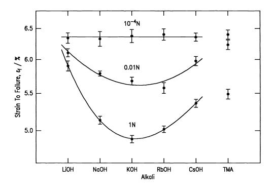
Fig. 4. Strength as a function of hydroxide for three different concentrations and a face plate velocity of  $100\mu m.s^{-1}$ .
