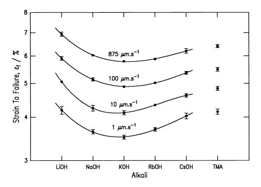
Fig. 3. Strain to failure as a function of 1N alkali solutions for four different face plate velocities.
