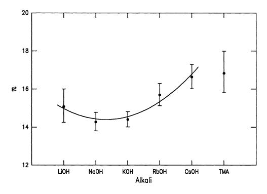
Fig. 6. Stress corrosion parameter, n, as a function of alkali for dynamic fatigue in 1N solution.
