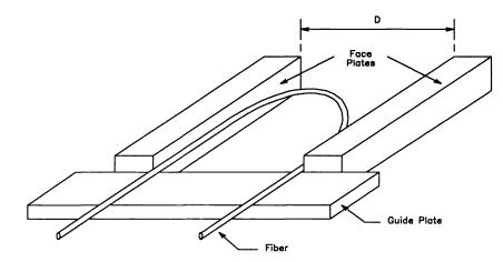
Fig. 2. Schematic of the two point bend apparatus for determining fiber strength.
