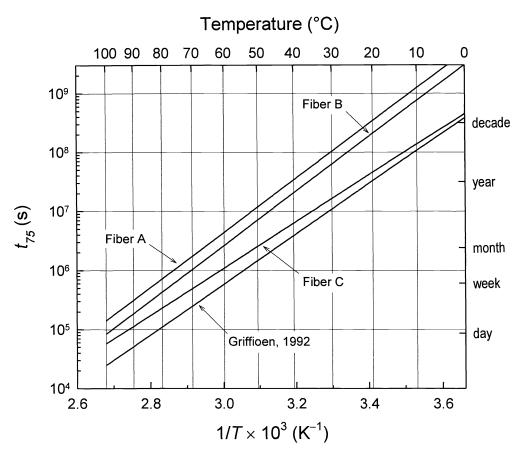
Fig. 5. Arrhenius plot of the values of the time for 25% strength reduction,  $t_{25}$ , from the fits to the data of Figs. 1 to 4.
