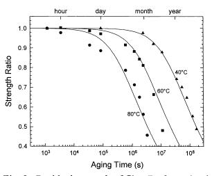
Fig. 2. Residual strength of fiber B after aging in deionized water.
