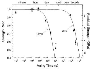
Fig. 1. Residual strength of fiber A after aging in distilled water.
