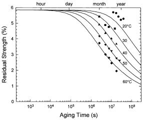
Fig. 4. Data of Griffioen<sup>3</sup> for residual strength (strain to failure) of fiber aged in water.
