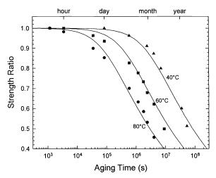
Fig. 3. Residual strength of fiber C after aging in deionized water.
