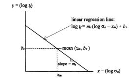
Figure 2. Schematic of linear regression model for fitting static fatigue data.
